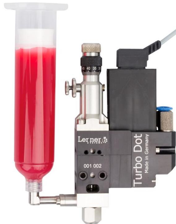
The TD118 electro-pneumatic high-performance jet valve is designed for the contactless microdispensing of low and medium viscosity fluids. A micro-dosing volume of 2nL or larger can be dispensed at frequencies as high as 280 Hz. Allowing the valve to dispense single dots as well as lines. The definable dot sizes range from 0.3 mm up to 5.0 mm in diameter depending on the media. Dispensing distances between valve and component are usually within 0.5 mm and 10.0 mm.
