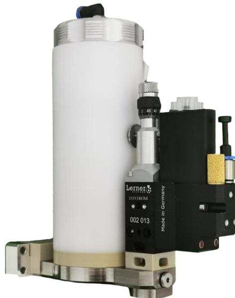
The TD118HM electro-pneumatic high-performance jet valve is designed for the contactless microdispensing of hot melt adhesives. A micro-dosing volume of 2nL or larger can be dispensed at frequencies as high as 280 Hz. Allowing the valve to dispense single dots as well as lines. The definable dot sizes range from 0.3 mm up to 1.5 mm in diameter depending on the media. Dispensing distances between valve and component are usually within 0.5 mm and 3.0 mm.
