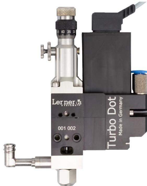
The TD118SP electro-pneumatic high-performance jet valve is designed for the contactless microdispensing of Type 5-7 solder pastes. The definable dot sizes range from 0.35 mm up to 1.5 mm in diameter depending on the solder paste. They can be dispensed at frequencies as high as 170 Hz. Allowing the valve to dispense single dots as well as lines. Dispensing distances between valve and component are usually within 0.5 mm and 3.0 mm.
