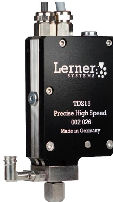
Our high-performance jet valves are designed for a contactless microdispensing of Type 5-7 solder pastes. The definable dot sizes range from 0.2 mm up to 1.5 mm in diameter and can be dispensed at frequencies as high as 500 Hz depending on the media. Allowing the valve to dispense single dots as well as lines. Dispensing distances between valve and component are usually between 0.5 mm and 3.0 mm.
